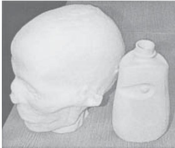
Reconstruction of Egyptian mummy, and detergent bottle made by 3-D printer.
