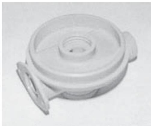
A prototype pressure vessel lid with valve housing made by SLA process
