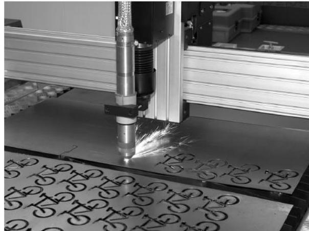
The laser is positioned by motors A and B which are operated by a microcontroller.
