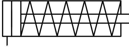
A Single-acting cylinder requires only one air supply. When air is put into the cylinder it **outstrokes**. After the cylinder has been de-activated it **instrokes** automatically, because of the spring.
