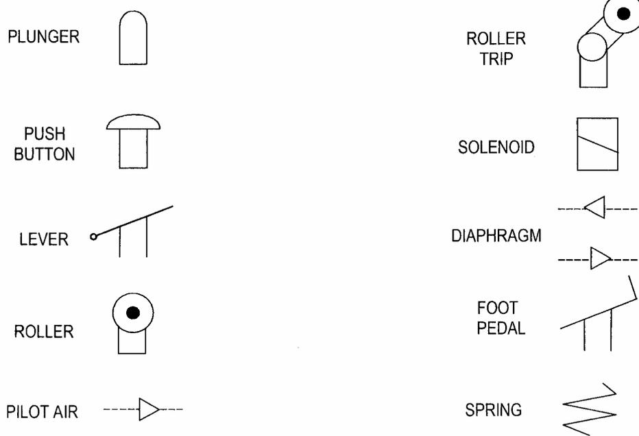
There are a number of different ways we can operate a 3/2 valve. The most common types of actuators are shown above
