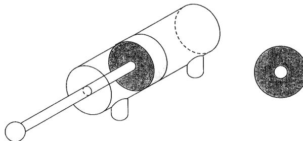
We can find this surface area or *effective area*, as calculating the area of the piston rod and subtracting it from the area of the piston know it.
