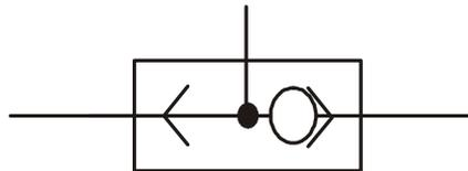
A shuttle valve is used to change the direction of air in a circuit. It has a small ball inside that gets blown from side to side.
