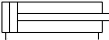
A double-acting cylinder has no spring inside to return it to its original position; *it needs two air supplies, one to outstroke and one to in stroke the piston.*
