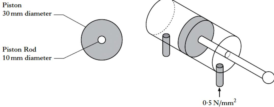
(c) Calculate the in-stroking force.
