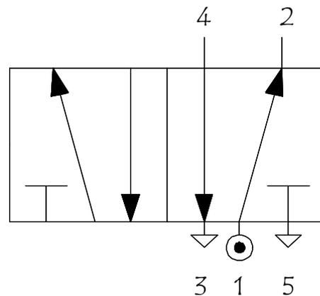
Another disadvantage is that the 3/2 valve needs to be actuated until the cylinder is fully out/in stroked. Releasing the valve will mean the piston will stop short of its final position.
