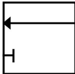
When naming the component you have to state its FULL name. For example this one would be known as a 'Roller Trip Actuated, 3/2 Valve, Spring Return'
