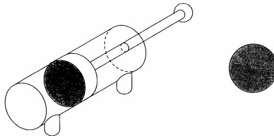
However, during the in stroke the surface area is reduced because of the piston rod. This means that the compressed air does not have as big an area to push against and so it does not produce as big a force.
