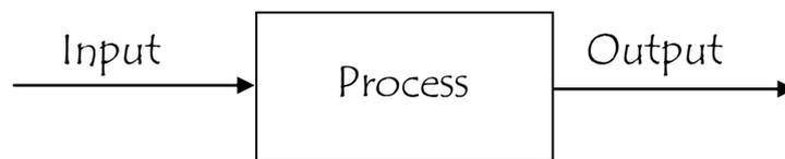
This block diagram is called the UNIVERSAL SYSTEM and can be applied to any system.
