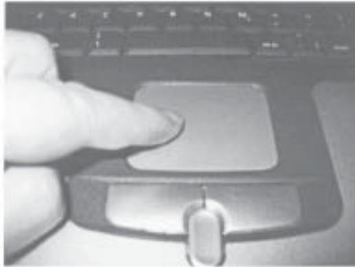
Beneath the surface there are two layers that together create an electromagnetic field. When an object such as a finger touches the surface the properties of the electromagnetic field change and the details are input to the computer.
